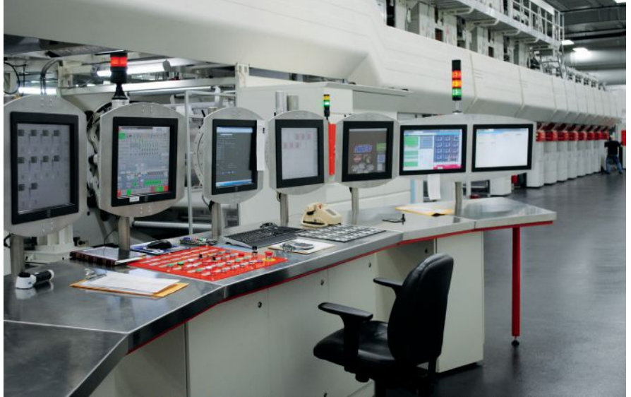
One of American Packaging Corporation's press operator command centers, including a 100 percent defect detection system.
